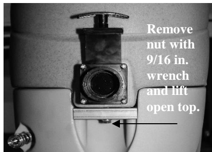
FIG. 4: Solution inlet filter cleaning
