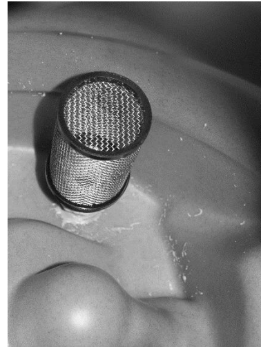
FIG. 6: Recovery tank strainer
