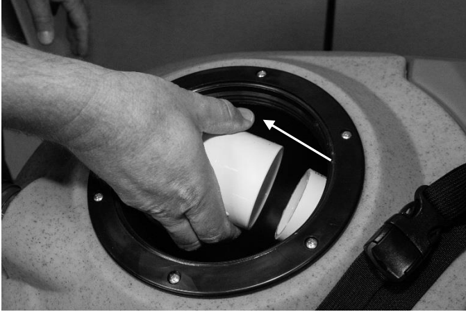
FIG. 5: Vacuum cutoff valve cleaning
