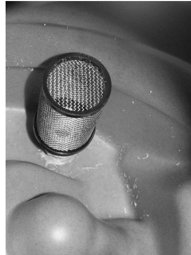
FIG. 6: Recovery tank strainer
