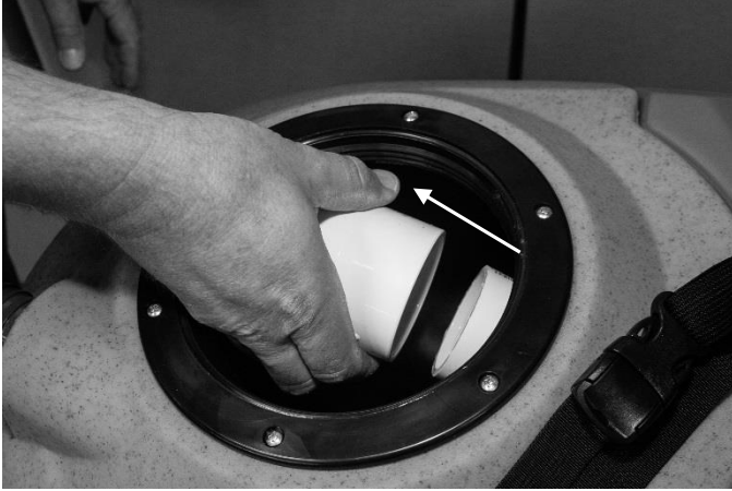
FIG. 5: Vacuum cutoff valve cleaning
