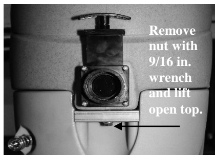
FIG. 4: Solution inlet filter cleaning
