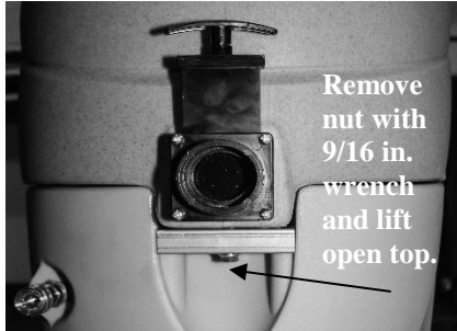
FIG. 4: Solution inlet filter cleaning
