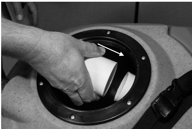
FIG. 5: Vacuum cutoff valve cleaning
