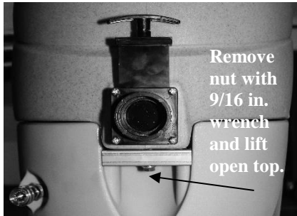
FIG. 4: Solution inlet filter cleaning
