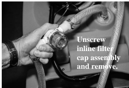
FIG. 4: Solution inlet filter cleaning
