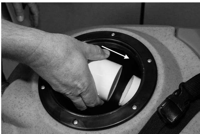
FIG. 5: Vacuum cutoff valve cleaning
