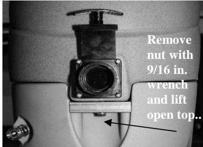
FIG. 4: Solution inlet filter cleaning
