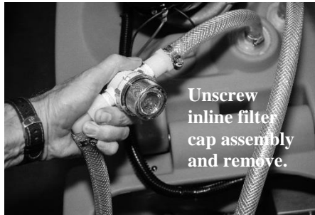
FIG. 4: Solution inlet filter cleaning
