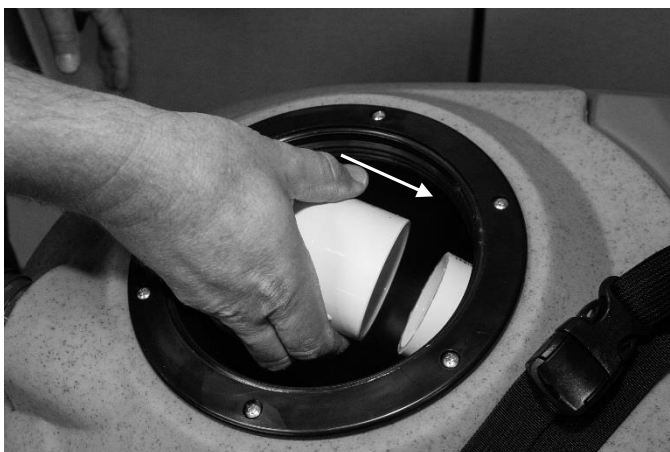
FIG. 5: Vacuum cutoff valve cleaning
