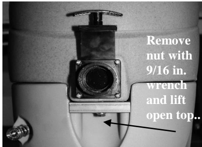
FIG. 4: Solution inlet filter cleaning
